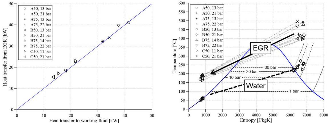
**Figure 5:** Heat transfer in the EGR boiler (left) and T-s diagram comparing fluid and EGR temperatures (right) at various ESC operating points and boiling pressures without an EGR after-cooler
