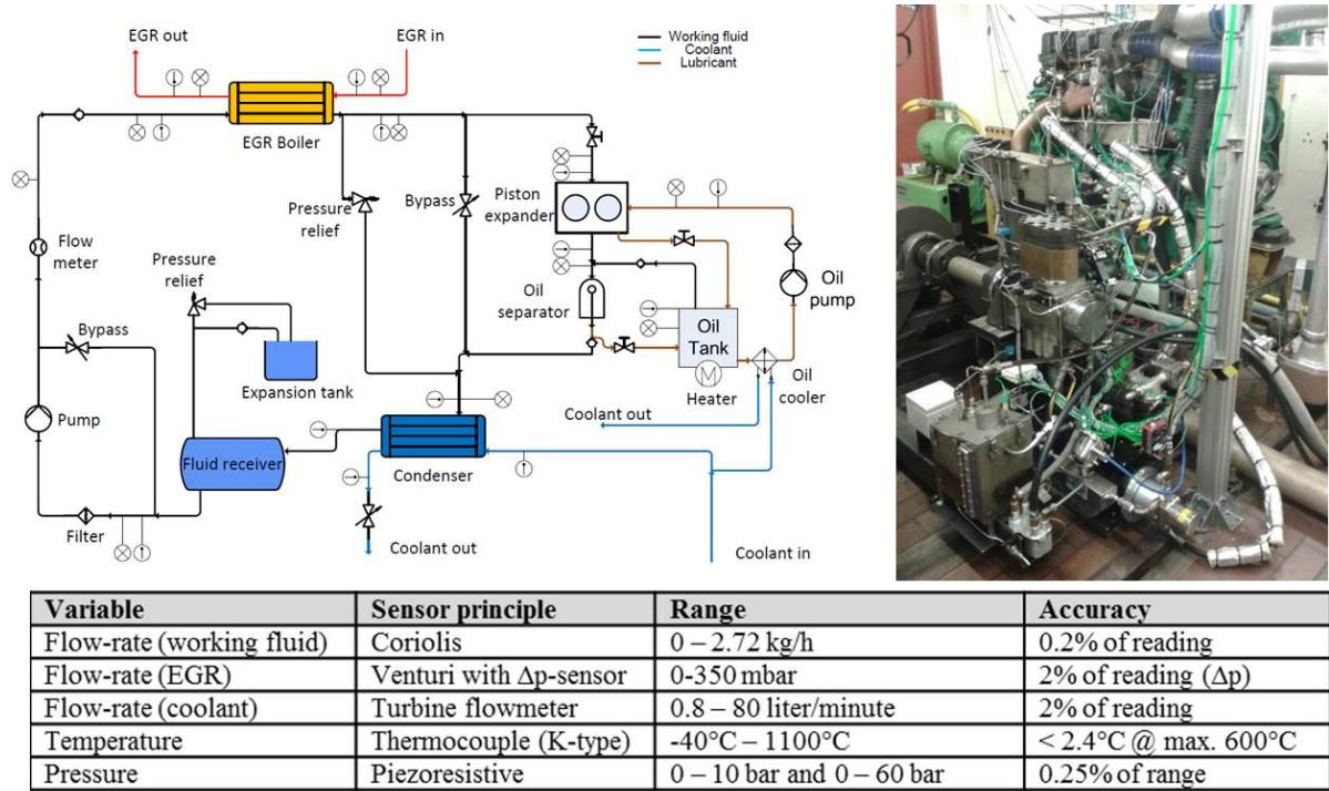
**Figure 1:** Experimental system layout and specification of the measurement equipment
