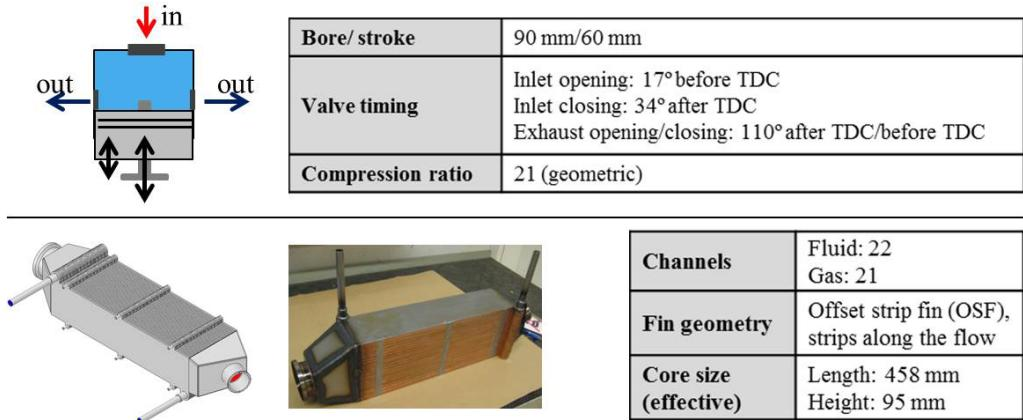
**Figure 2:** Schematic diagram and geometry of the uni-flow expander (upper image and table) and the EGR boiler (lower image and table)
