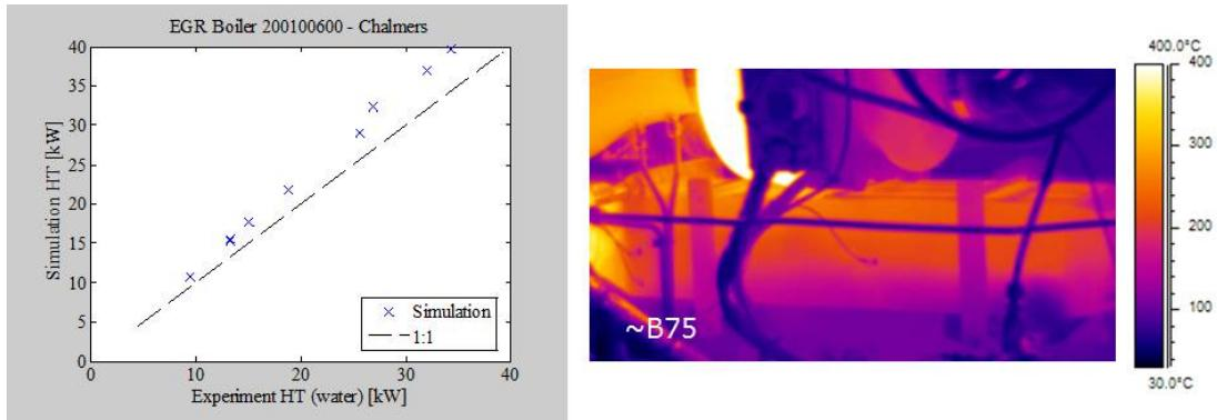
**Figure 9:** Comparison of simulation and experimental data (left). Engine load varies between A25 and B75, hence flows and pressures of both EGR and water also vary. Infrared image of the boiler side-plate (right). Fluid enters at the bottom right corner and exits at the top left corner. EGR flows from left to right.
