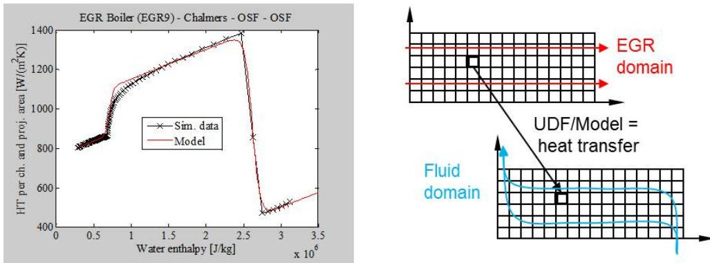
**Figure 4:** UDF (“Model”) describing projected heat transfer per channel and projected plate area. The principle of the UDF is illustrated by the figure to the right, showing CFD representations of an EGR- and a fluid channel.
