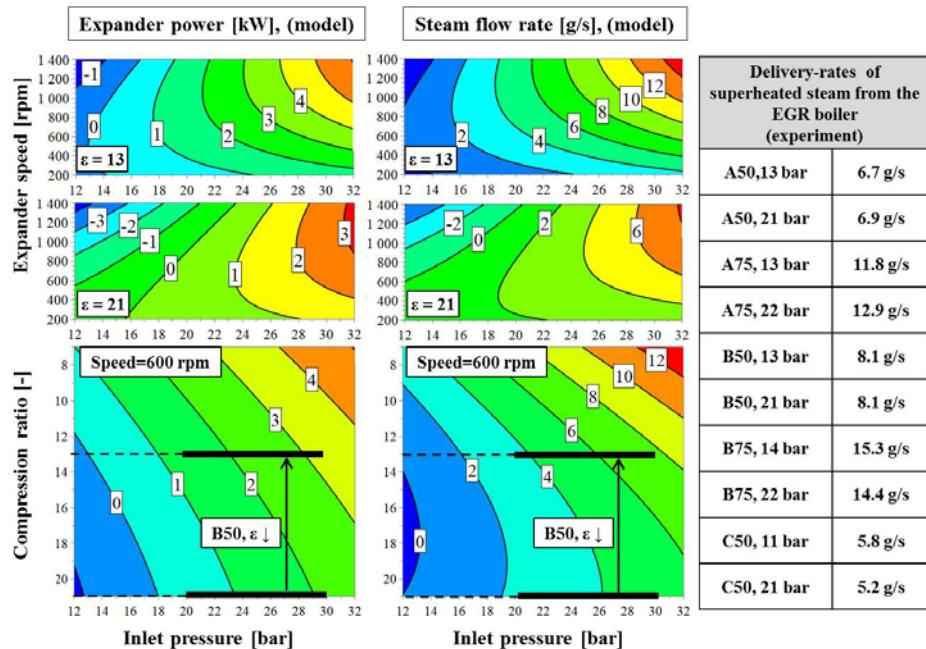
**Figure 8:** Modeled expander power and steam flow rate as functions of expander speed, compression ratio  $\epsilon$  and inlet pressure (left). List of measured steam-delivery rates of the EGR boiler prototype (right).
