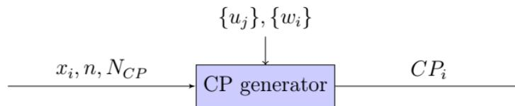
**Figure 2: Interpolation algorithm.**  $x_i$ ,  $n$  and  $N_{CP}$  are the data points, the degree of the B-Spline curve and the desired number of control points, respectively.  $\{u_j\}$  and  $\{w_j\}$  are the knot sequence and the data parameters. As output, the control points  $CP_i$  of the B-Spline are generated.
