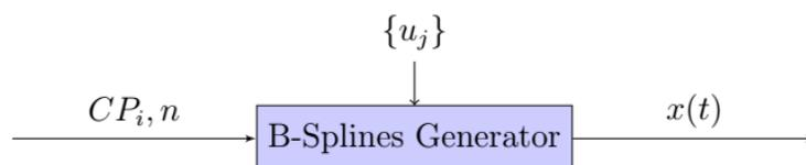
**Figure 1: Geometry generation algorithm.**  $CP_i$  and  $n$  are the control points and the degree of the curve, respectively;  $\{u_j\}$  is the knot sequence. As output, the B-Spline curve  $x(t)$  is generated.
