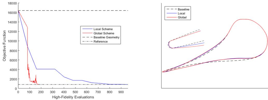
**Figure 4: Left: convergence history of global and local strategies for surrogate-based optimization. Right: optimized geometry using global and local strategies for surrogate-based optimization.**
