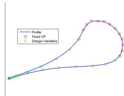
**Figure 3: Baseline profile shape and control points distribution. Green circles indicate design variables, while red ones are kept fixed during optimization. The black circle indicates de control point that moves accordingly to keep the trailing edge width constant.**
