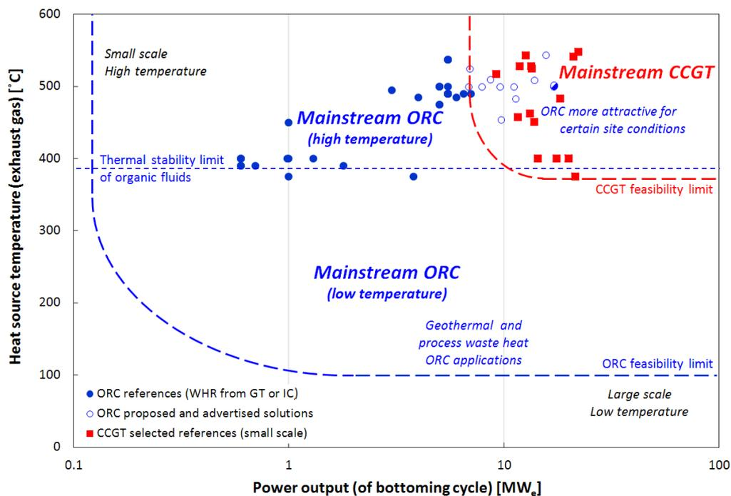
**Figure 5:** Heat source temperatures and power outputs for which ORC and CCGT systems are considered viable. This figure should only be used as an approximate indication; it was inspired by the figure from (Gaia,
