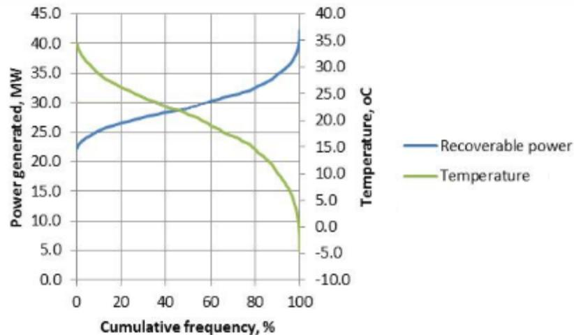
**Figure 4:** Temperature distribution and accompanying ORC power output. The yearly average recoverable electric power is estimated at 29.6 MW<sub>e</sub>.
