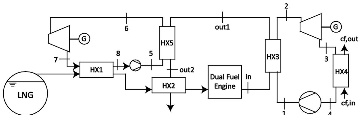
Figure 1: Dual loop ORC system for LNG carrier
