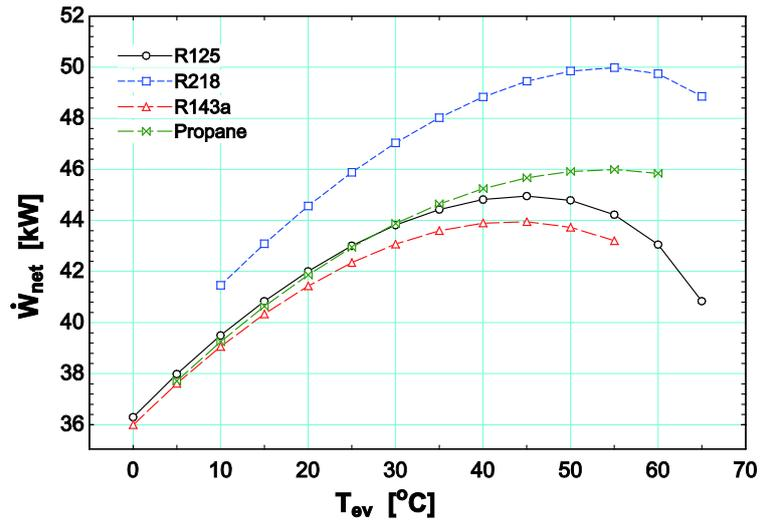
Figure 3: Power output of LT-ORC corresponding to evaporation temperature
