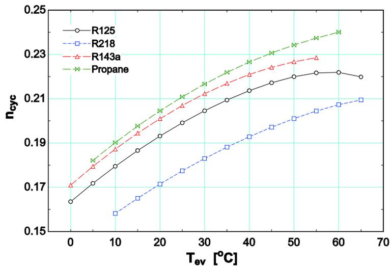
Figure 4: Cycle efficiency of LT-ORC corresponding to evaporation temperature
