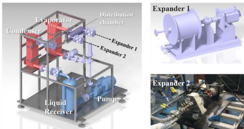
Figure 2: Schematics of ORC system and Expander 1, and a photograph of Expander 2
