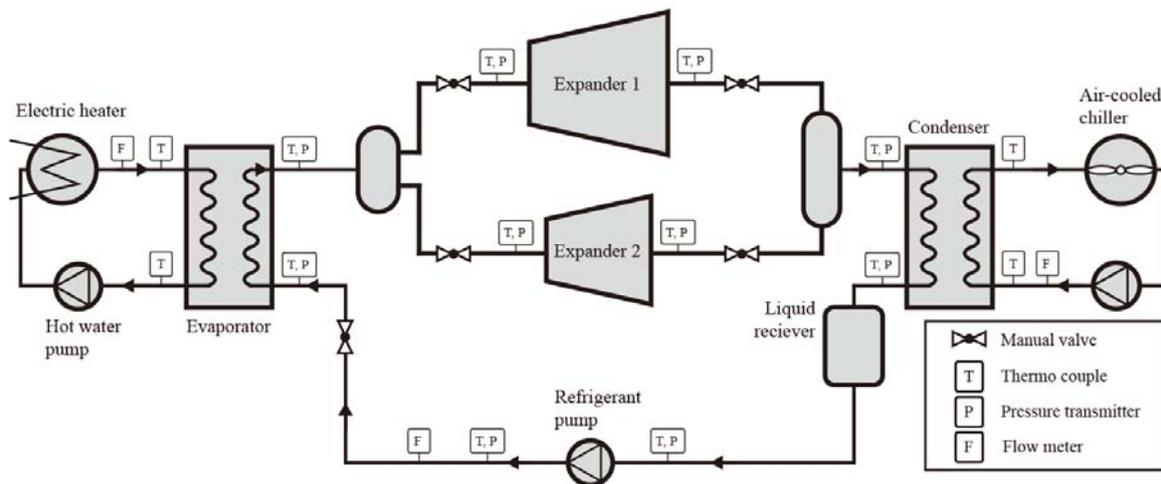
Figure 1: Schematic diagram of Dual-expander ORC test rig
