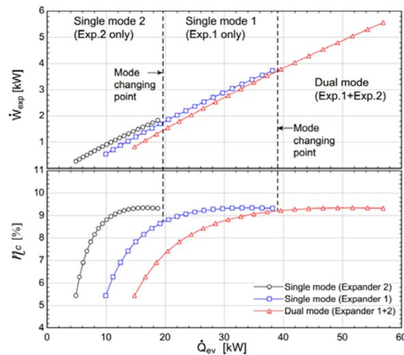
Figure 5: Predicted power outputs and cycle efficiencies for three operating modes (Single modes and Dual mode) and mode changing points for maximizing cycle efficiency
