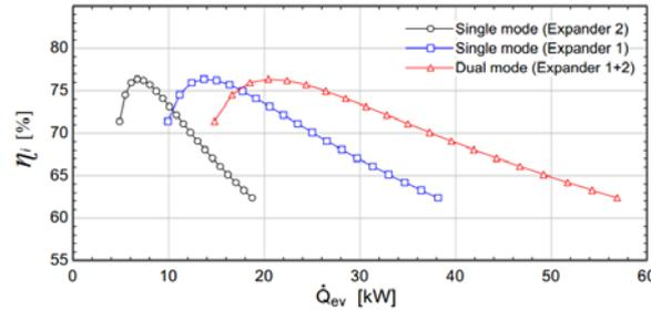
Figure 4: Predicted isentropic efficiencies for three operating modes (Single modes and Dual mode)
