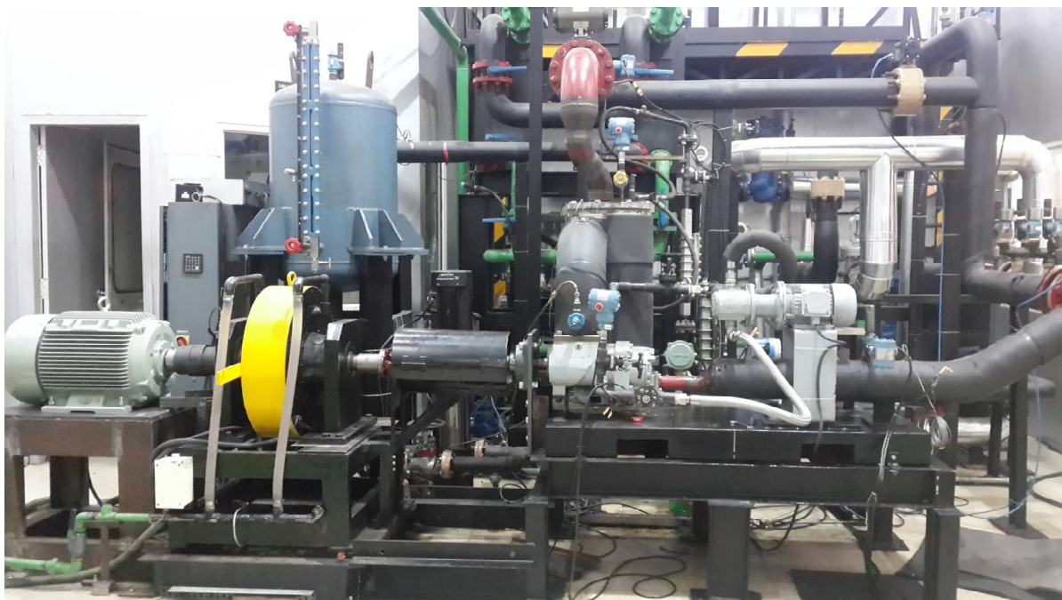
Figure 1: ORC test facility (with screw expander)
