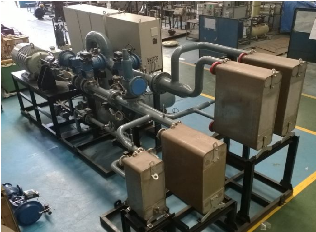
Figure 7: First prototype of ORC system: Capacity 100 kW
