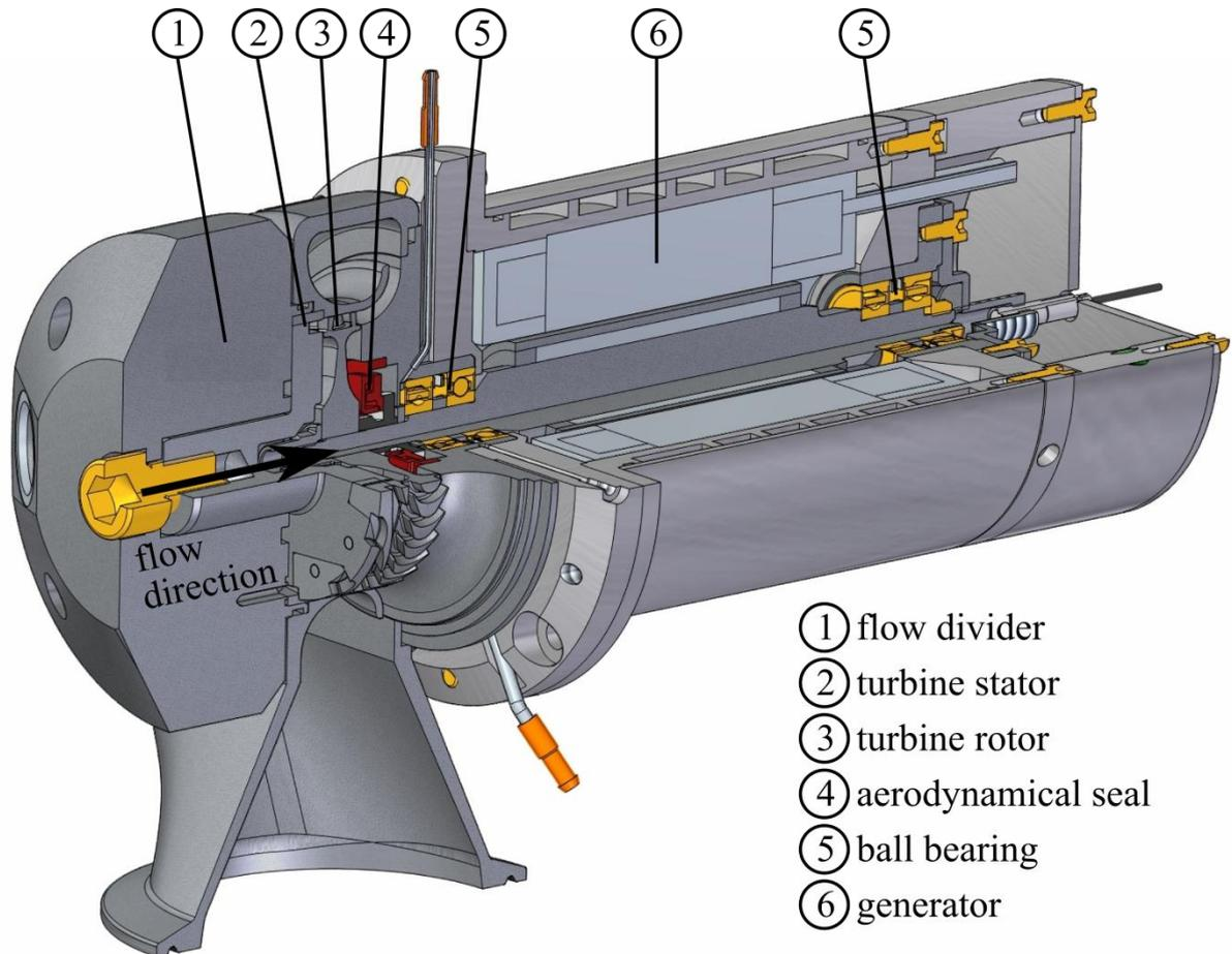
Figure 4: Mechanical design of the expansion machine
