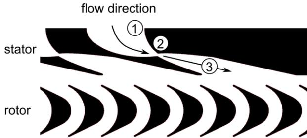
Figure 2: ORC Blade profile of the turbine
