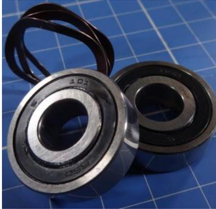
Figure 6: Ball bearings and spring
