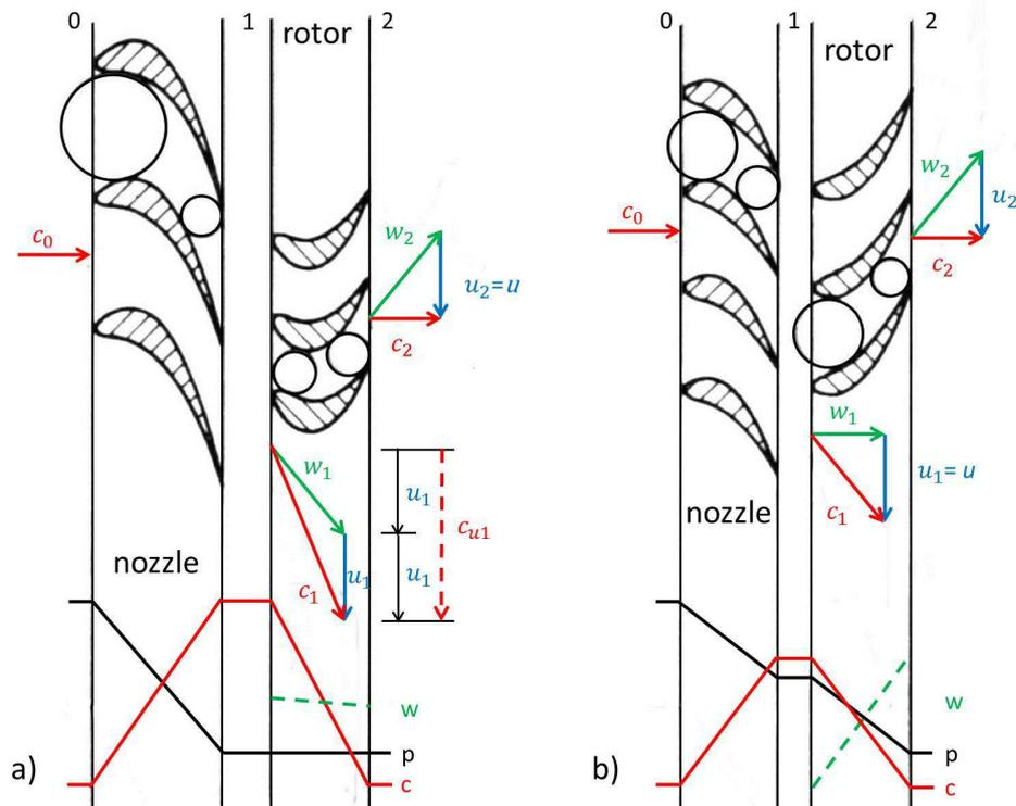
Figure 3: Comparison impulse (a) and reaction stage (b)
