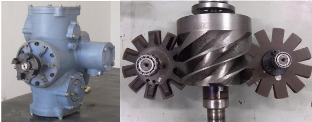
Fig.1: Photograph of the single-screw expander
