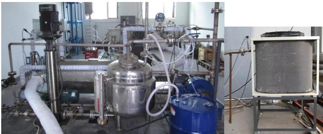
**Fig.2:** ORC system prototype
