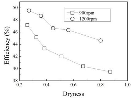
**Fig.10:** Power output versus inlet vapor dryness **Fig.11:** Shaft efficiency versus inlet vapor dryness
