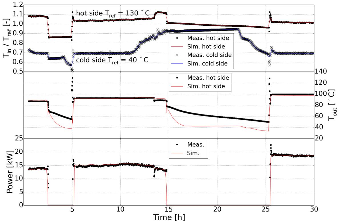
**Figure 9: Top: Normalized water temperatures at the evaporator and condenser inlet. Middle: Measured and simulated water temperatures at the evaporator outlet. Bottom: Measured and simulated gross electrical power of the ORC module.**
