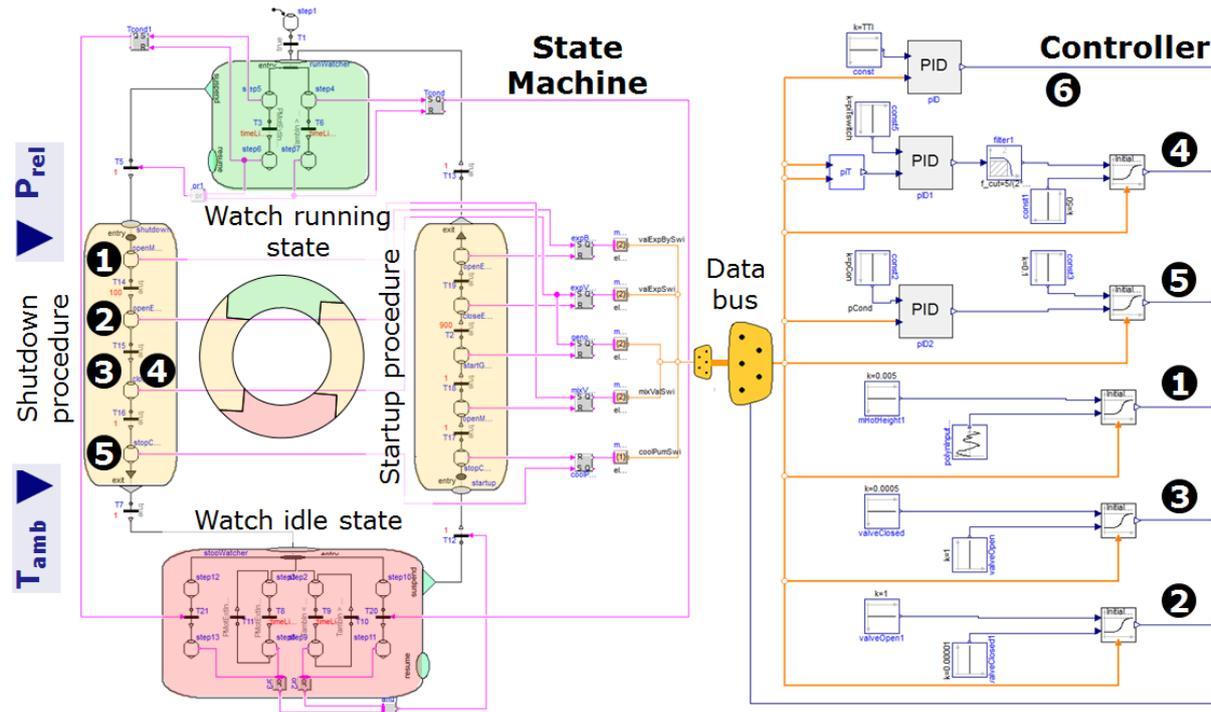
**Figure 4: The control strategy consists of a state machine coupled with a controller. The numbers in the state machine and controller section correspond to the process data and actuators depicted in Figure 3.**
