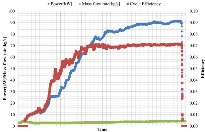
Figure 7: Power and efficiency change during startup
