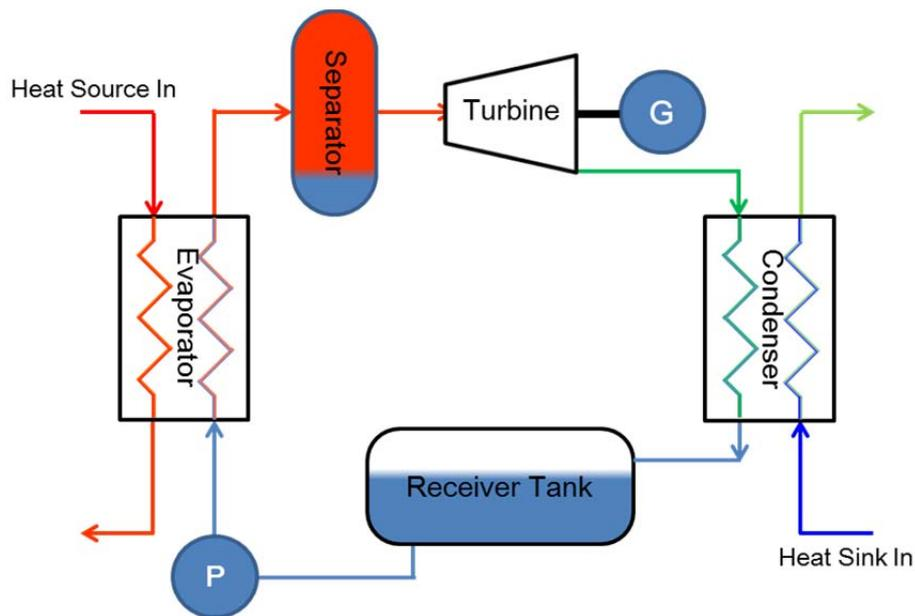
Figure 2: Schematic diagram of ORC power generator
