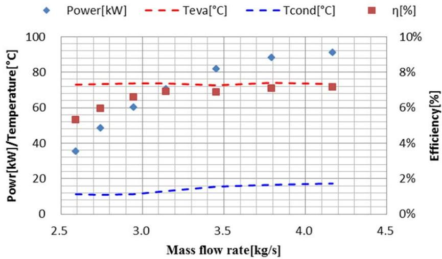
Figure 8: Performance results of 100kW ORC generator
