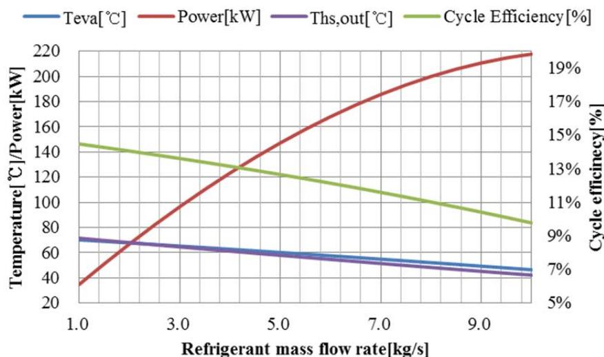
Figure 1: Effects of working fluid flow rate
