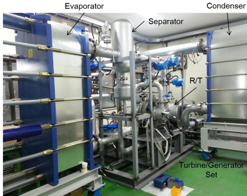
**Figure 6:** Photo of a 100kW Geothermal ORC Turbo-generator
