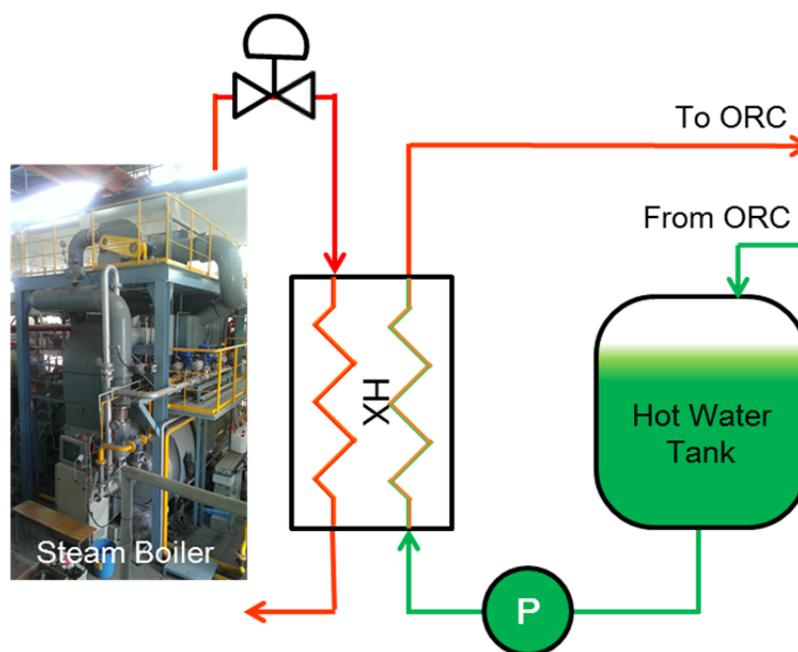
**Figure 5:** Schematics of hot water supply system
