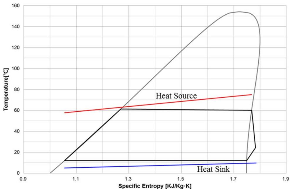
Figure 3: T-s diagram of the present ORC cycle
