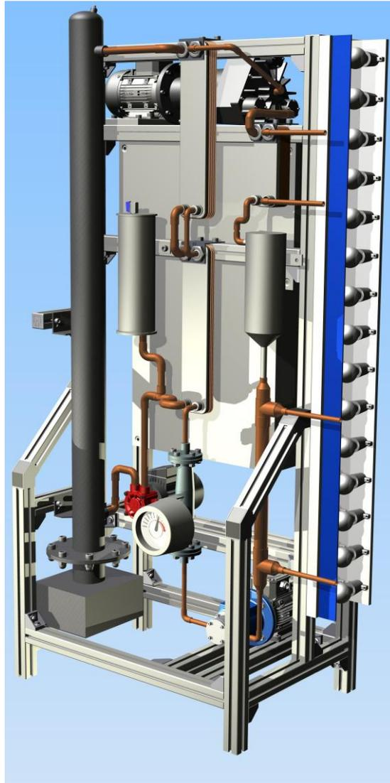
**Figure 3:** Design of the 1 kW ORC demonstration plant
