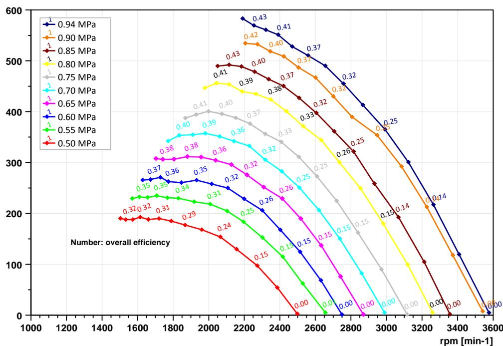
Figure 6: Electric Power versus rpm with overall efficiency
