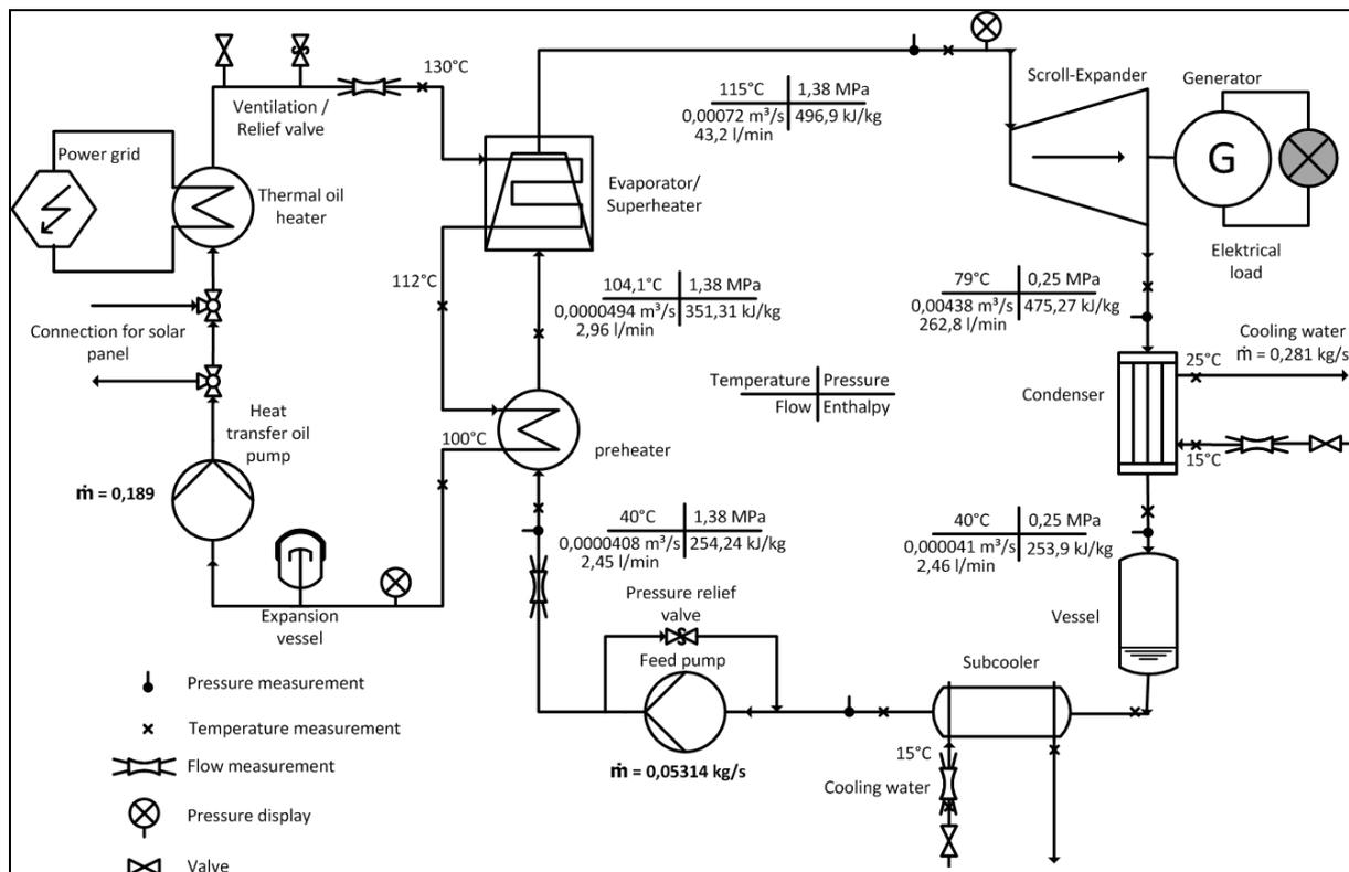
Figure 1: ORC demonstration plant – connection schema
