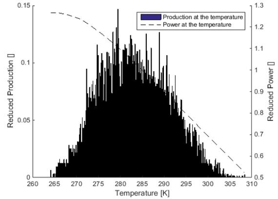
**Figure 6: Reduced power and contribution to production vs ambient temperature**
