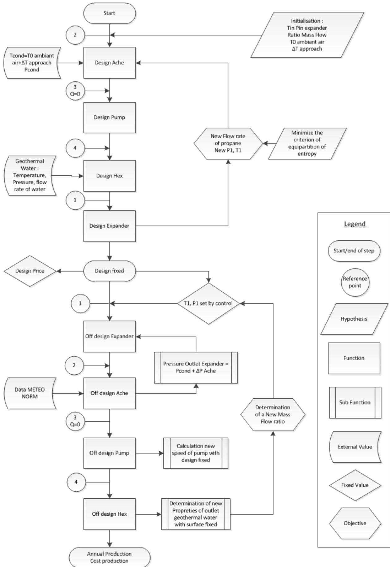
Figure 4: Algorithm logic diagram
