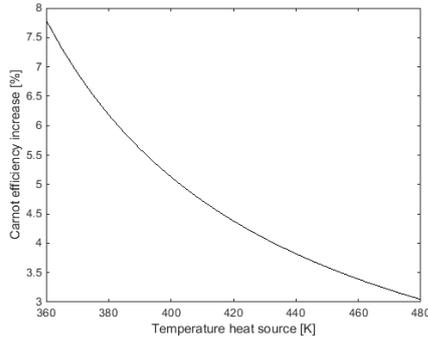
$$f(T_{hot}) = \frac{(1 - \frac{277}{T_{hot}}) - (1 - \frac{283}{T_{hot}})}{1 - \frac{283}{T_{hot}}} * 100 \quad (1)$$
