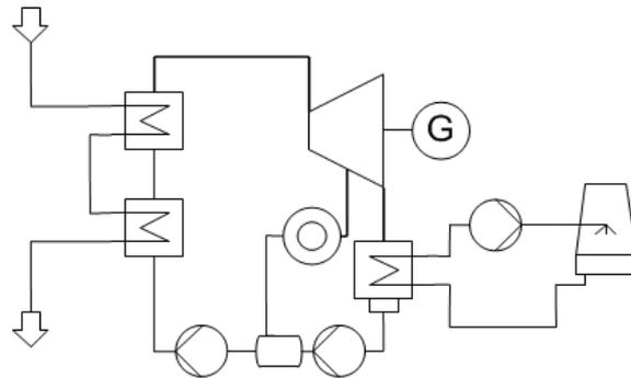
**Figure 5:** Integrated CHP concept with regenerative pre-heating
