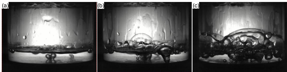
Figure 4: Visualization for water with smooth surface. (a) v_{p,max} = 8 mm/s, (b) v_{p,max} = 32 mm/s and (c) v_{p,max} = 128 mm/s.
