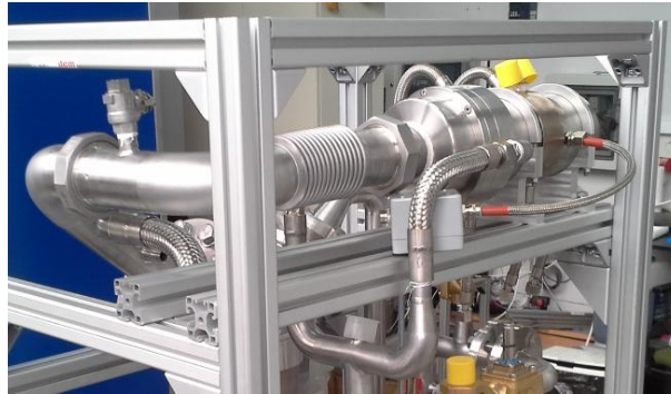
Figure 2: Photo of turbo-generator mounted on the frame of the micro power plant
