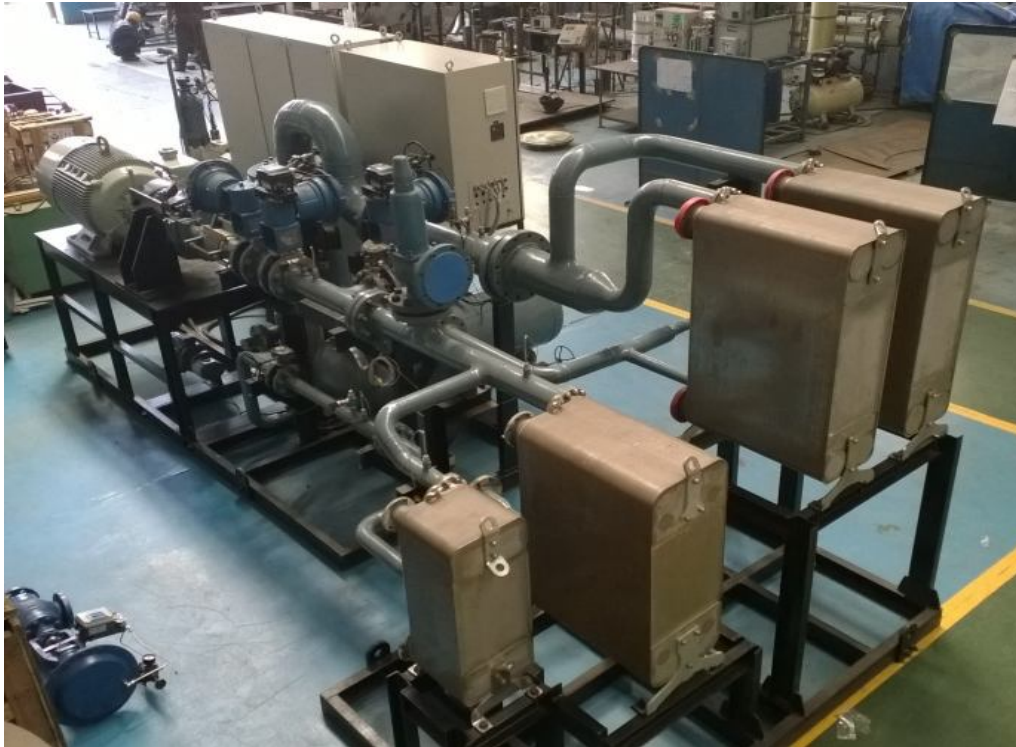
Figure 7: First prototype of ORC system: Capacity 100 kW
