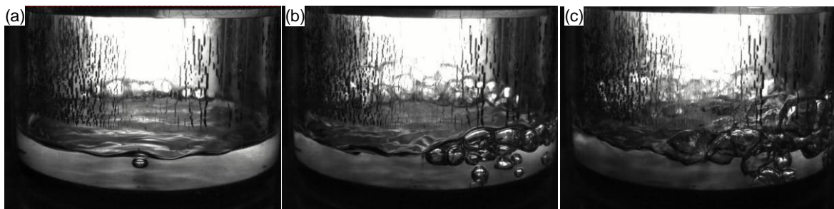
Figure 5: Visualization for ethanol with smooth surface. (a) v_{p,max} = 8 mm/s, (b) v_{p,max} = 32 mm/s and (c) v_{p,max} = 128 mm/s.
