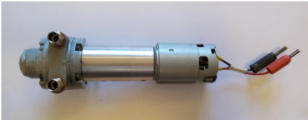
Figure 2: The view of the expander-generator unit disassembled from the test-stand
