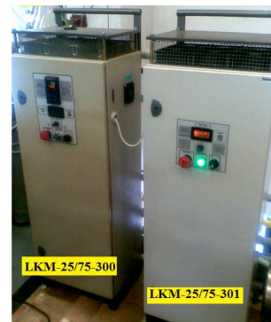
Figure 5: Prototype electric flow heater for thermal oil
