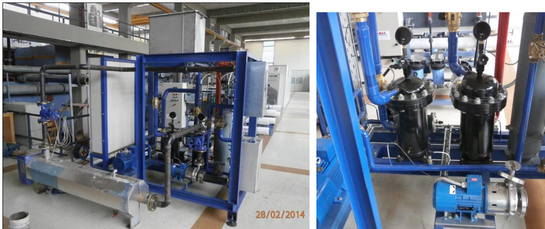
Figure 2: The integrated system installed in the laboratory and the scroll expanders
