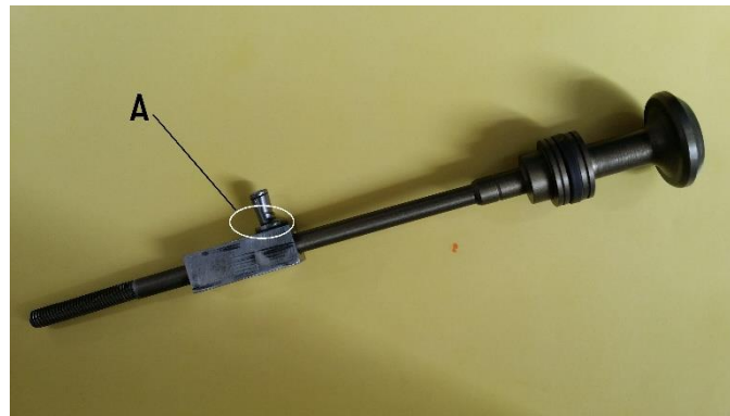
Figure 9: Actual failure region of the inlet valve slider
