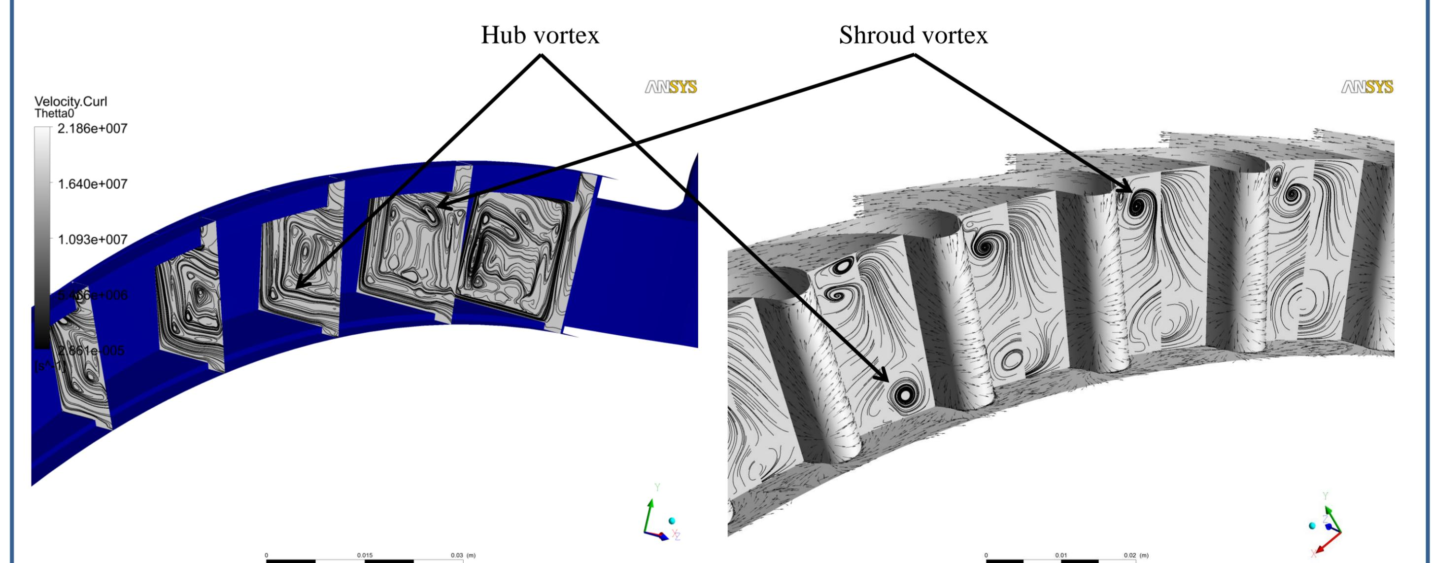
➤ Specific shape of the shock wave after the blade wheel. The intensity of the normal shock wave decreases from hub to shroud. Shroud vortex is underexpanded and continues its expansion after the blade wheel
