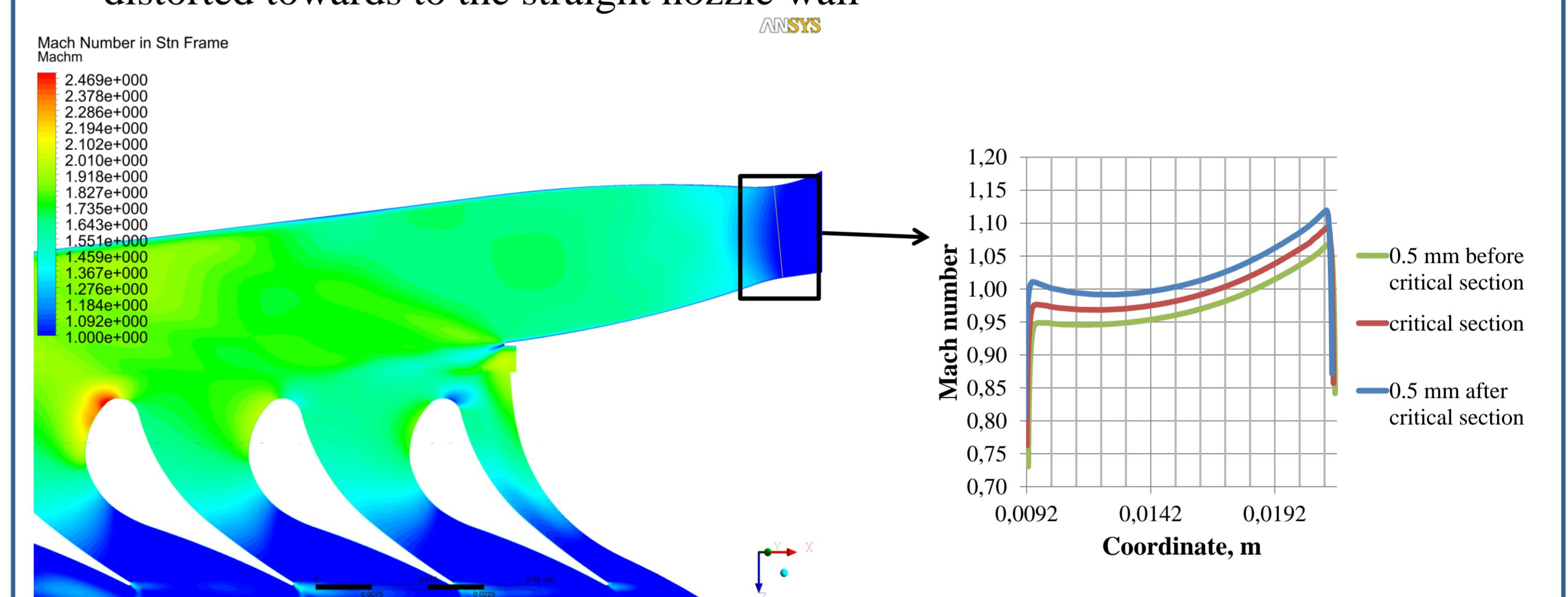
➤ The double-vortex structure appears in the nozzle and spreads to the blade wheel. The hub vortex rotates clockwise and rests against the blade wheel hub. The shroud vortex has a counterclockwise rotation and rests against the blade wheel shroud because of the inertial forces
