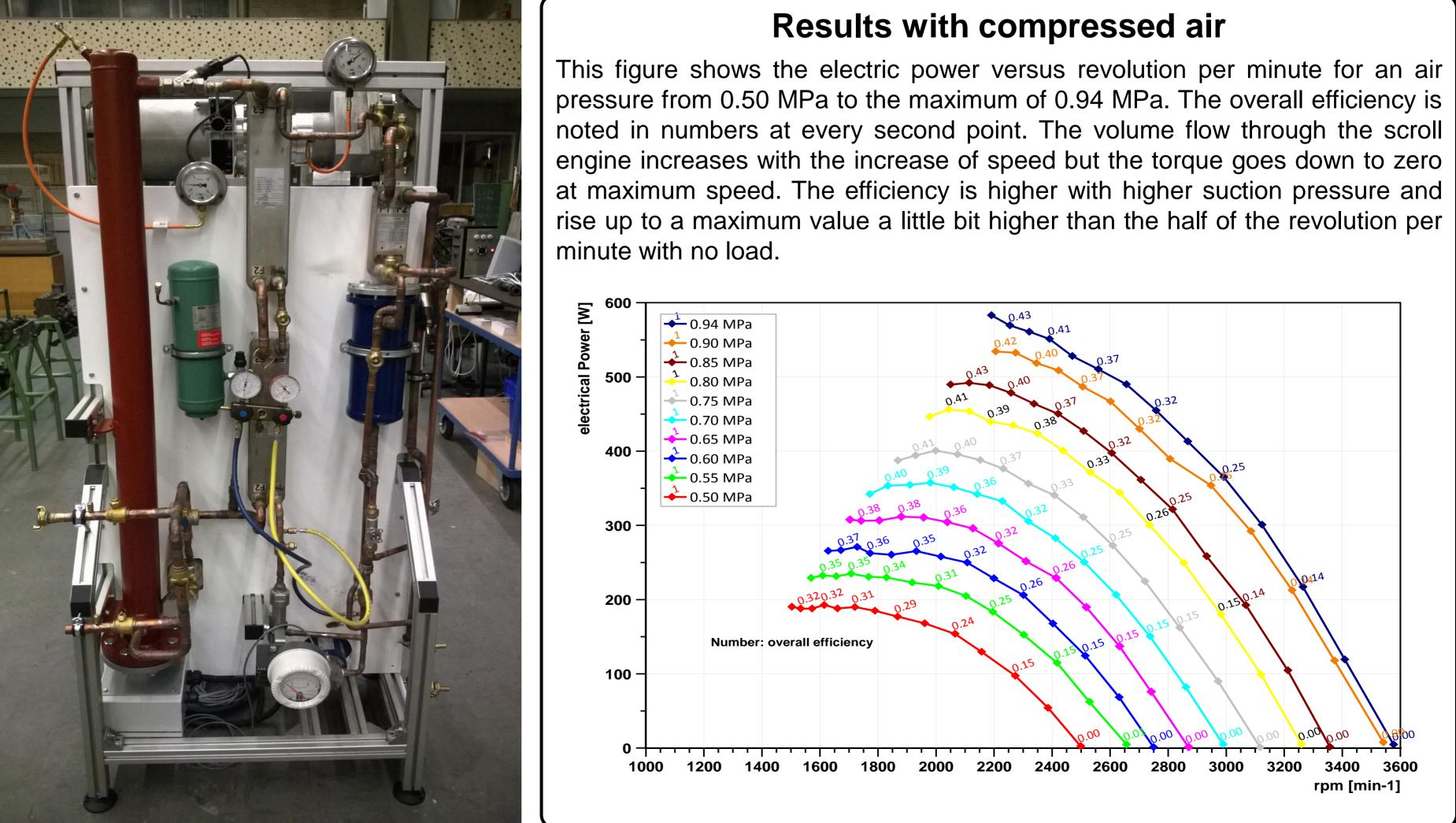
The software searches for the measured temperature and pressure the values for enthalpy and entropy to the main condition points from a table. Additional to the heat power, the electrical power, the revolution and the efficiency these points are also visualized in a h-s-diagram and a T-sdiagram.
