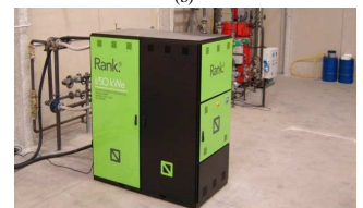
Figure 4: ORC modules: (a) Power generation system integrated in the industrial application, (b) CHP system during tests, (c) Power only and CHP system during tests.
