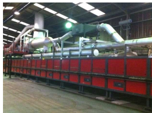
Figure 1: Industrial furnace of Keros Ceramica and heat recovery facility: (a) heat transfer loop, (b) facility scheme.
