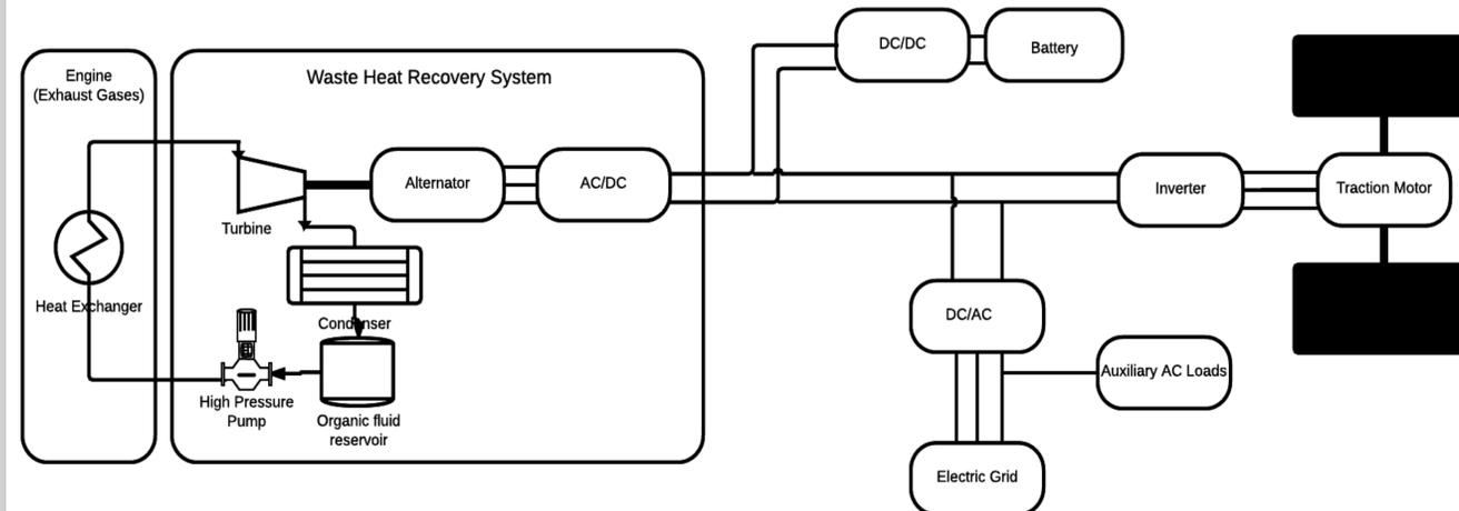
Figure 3: The ORC and Power Conversion Unit (PCU) architecture
