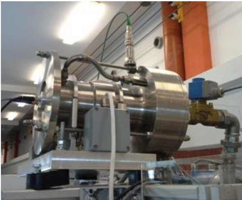
Turbogenerator with a radial-flow supersonic turbine
