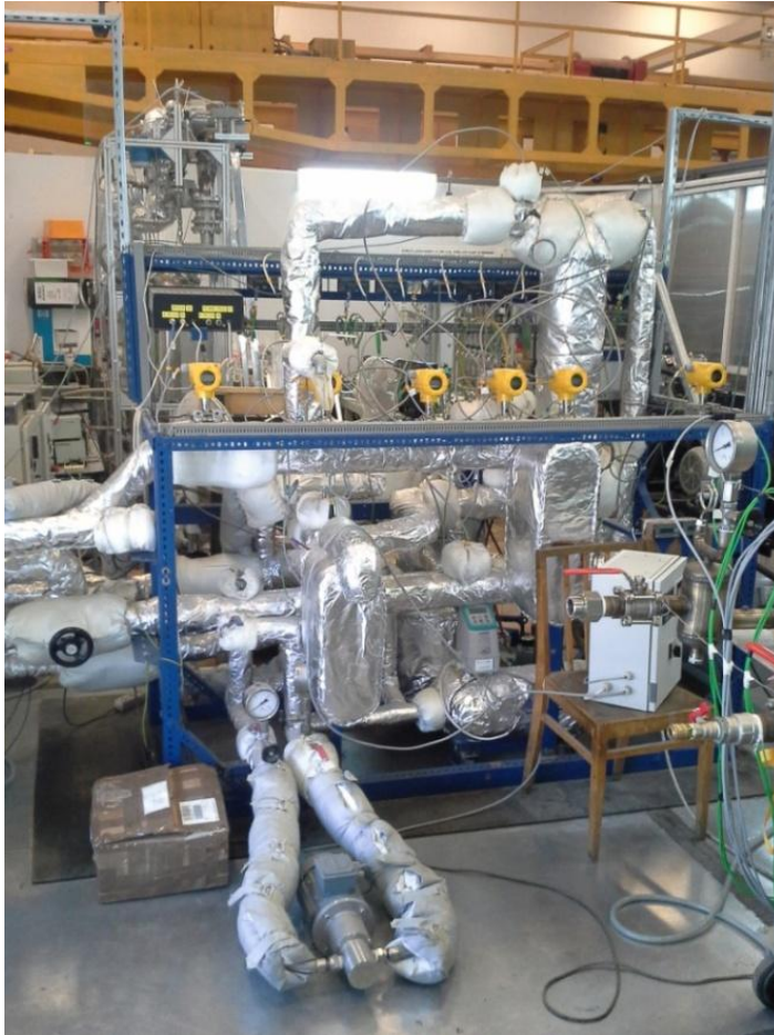
Test stand for testing heat exchangers
