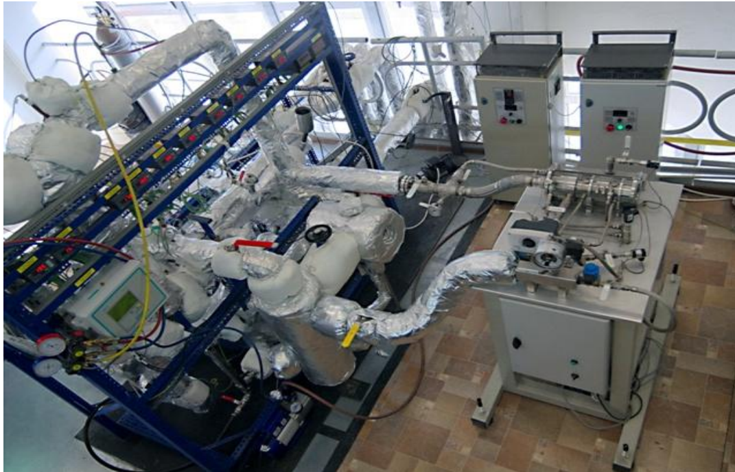
Testing of the heat exchangers and micro-turbine
