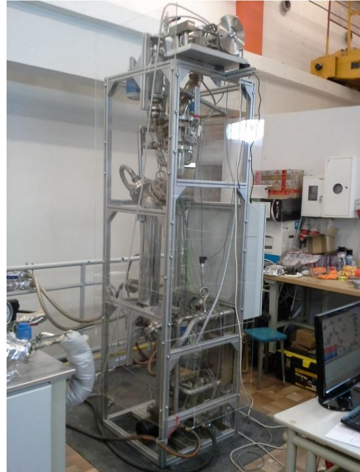
Test stand for testing micro power plant
