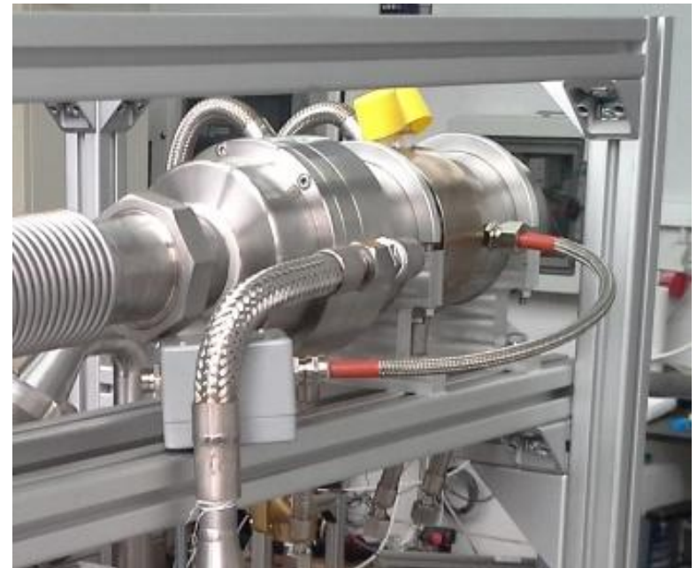
Turbogenerator with a radial-flow 4-stage turbine
