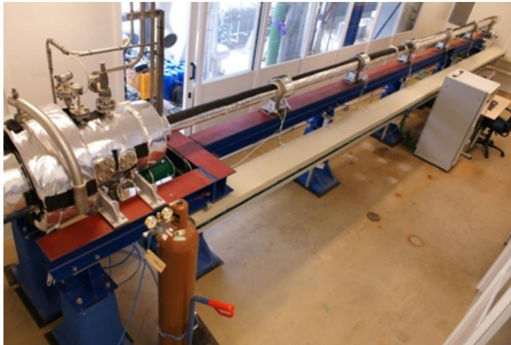
T. Mathijssen, M. Gallo, E. Casati, N.R. Nannan, C. Zamfirescu, A. Guardone, P. Colonna, "The flexible asymmetric shock tube (FAST): a Ludwieg tube facility for wave propagation measurements in high-temperature vapours of organic fluids", *Exp. In Fluids* 56:195, October 2015
