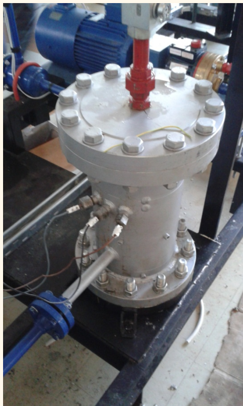
Top: Hermetic scroll expander and side view of ORC
