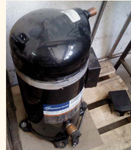
Hermetic scroll compressor (Copeland: ZP137- KCE-TFD)
