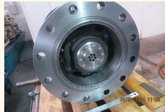
Hermetic scroll compressor (Copeland: ZP137- KCE-TFD)
