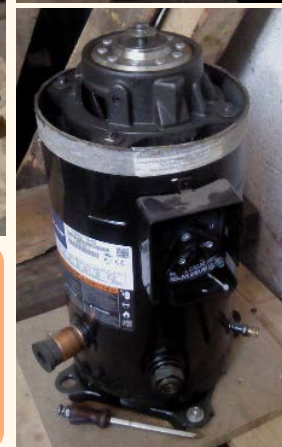
Hermetic scroll compressor (Copeland: ZP137- KCE-TFD)
