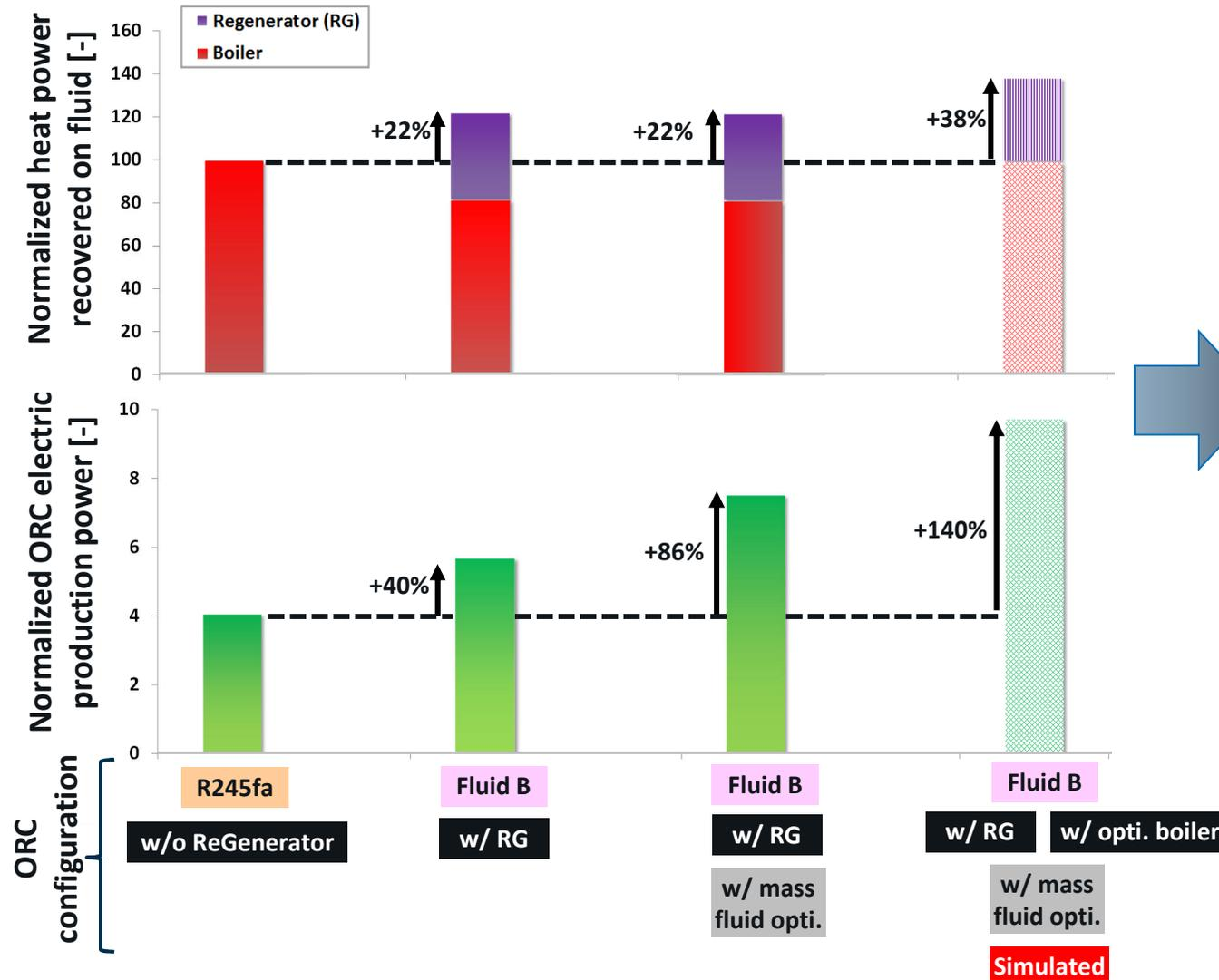
10kW of ORC electric production in steady-state conditions at the engine test bench for an objective of 14kW evaluated by simulation
